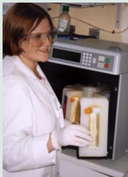
Fig. 10 Pamela McGarr conducting microwave preparation of otoliths prior to ICP-MS analysis.
