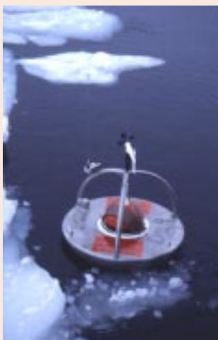
Fig. 48 Close-up of ice drifter with stainless steel casing to resist ice abrasion.
