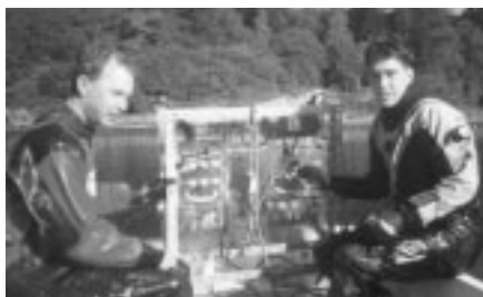
David Hughes (left) on fieldwork in Loch Sween, Argyll, with Jon Chamberlain, University Marine Biological Station Millport. The equipment (centre) is designed to measure the exchange of dissolved chemicals between the seabed and the overlying water.
