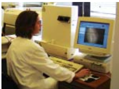
ICP-MS allows accurate measurements of a wide range of elements present in minute concentrations.
